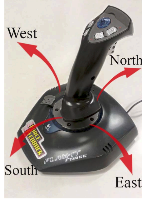
Fig. 2. The force-feedback (or tactile-force) joystick FLIGHT FORCE by Logitech used in experiments reported in this paper. The tactile-force stimulus was delivered to the subject's dominant hand. Four movements, defined as North , East , South and West directions, were executed randomly from a computer causing the joystick handle to move and push the subject's hand automatically.
