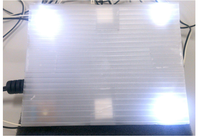
Fig. 2. Conventional monochromatic (ON-OFF) LEDs arrangement. In the experiments presented in this paper the following flashing frequencies were used: top-left 7 Hz; bottom-left 18 Hz; bottom-right 25 Hz; and top-right 39 Hz. The LEDs were arranged in the 7.4 \times 5.8 cm rectangular pattern. All LEDs are connected to ARDUINO UNO micro-controller board which generated four square waves with different frequencies.
