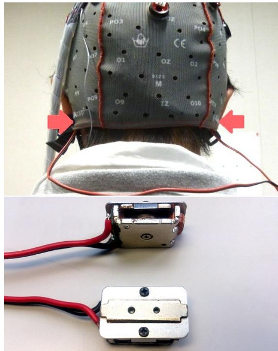
Figure 1. The experimental bone-conduction stimulus delivery set up. Each bone-conducting transducer (as shown in the lower panel) was set between each mastoids and the EEG cap surface. The top panel in the above figure depicts the transducer locations with red arrows. The bottom panel shows two BCT-1 22 x 14 mm bone-conducting transducers in top and side views. The same set up was used for the psychophysical and the EEG experiments.
