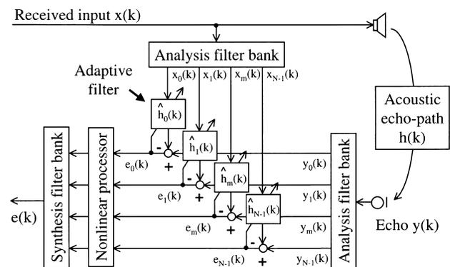
Fig. 1 Configuration of a subband echo canceller.
