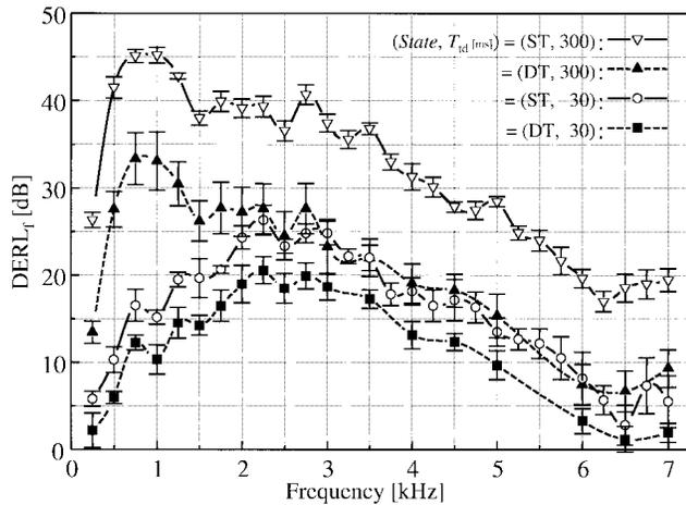
**Fig. 10** Subjective  $DERL_f$  test results for the differences between single-talk (ST) and double-talk (DT).
