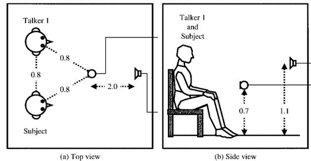
**Fig. 3** Top and side views of the assessment room layout (unit = meter).
