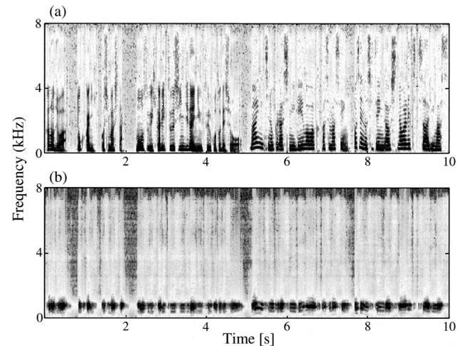
**Fig. 6** Spectrogram examples presented to the subjects: (a) near-end speech and (b) its band-limited echo.
