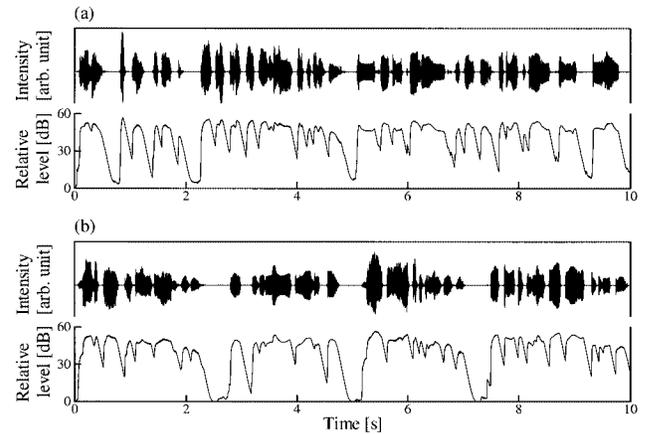
**Fig. 5** Waveforms and their power envelopes presented to the subjects: (a) near-end speech and (b) far-end speech.
