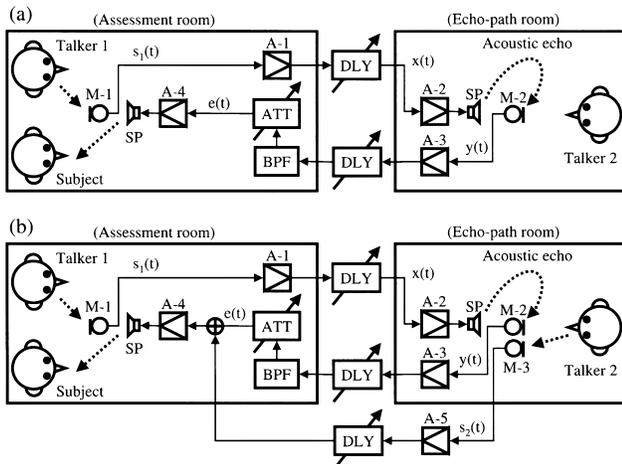
**Fig. 2** Schematic diagram of the subjective assessment system in (a) the single-talk state and (b) the double-talk state.
