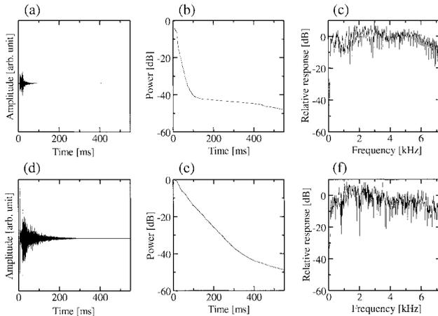
**Fig. 4** Impulse responses and acoustic characteristics of the echo-path room: (a), (b), (c) are impulse response, reverberation curve, and frequency response when  $T_{60}$  was 125 ms, (d), (e), (f) are those when  $T_{60}$  was 500 ms.
