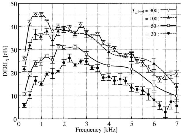
Fig. 7 Subjective  $DERL_f$  test results for transmission delays from 30 to 300 ms.
