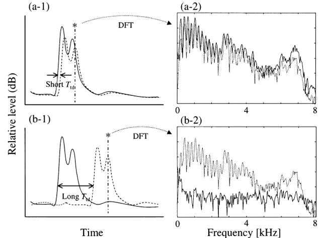
Fig. 8 Signal power envelopes and short-time spectra of the near-end speech (solid line) and its echo (dashed line) for different transmission delays.
