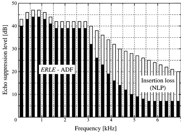
Fig. 11 Efficient subband echo canceller performance profile.
