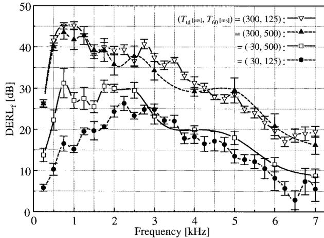
**Fig. 9** Subjective  $DERL_f$  test results for different reverberation times in the echo-path room.
