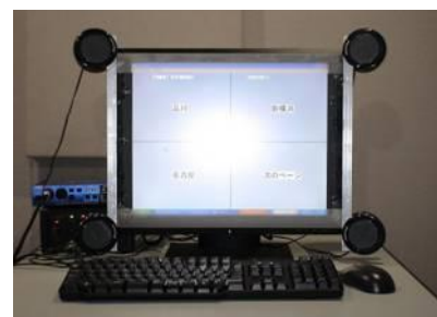
Fig. 4 Auditory interface by using sound localization
