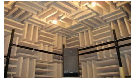
Fig. 2 Acoustic measurement in an anechoic chamber
